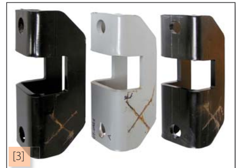
Result after 1000 h salt-spray test
